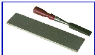
In order to really do good work with waterstones it is essential that you have a way of flattening stones. In a pinch a rough piece of wet or dry silicon carbide paper on a piece of glass will work, but a diamond stone is a lot easier to use.
