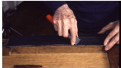
Notice how the follow-through of the stroke elevates slightly before it goes off the end of the strop. The whole arm raises, like an airplane taking off. Then replace the chisel at the beginning of the strop and strop again. During the contact part of this stroke the tool does not change angle. (The fragile, thin edge can actually be turned if firmly pressed out of true on the upswing.)
