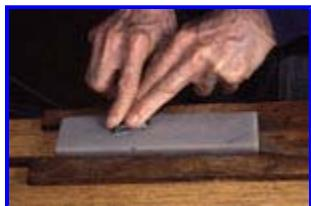
B. Rub the back of the tool perfectly flat on the Arkansas stone to remove any new burr raised in the prior step.
