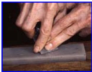
A. Rub bevel lightly on Arkansas stone with 5 degree increase in angle. Hold the chisel as before and then very slightly raise the back of the handle a minuscule amount with your pinky. It's hard to maintain a consistent angle with the handle raised so only move the chisel in one direction, then lift the chisel and return to start, and repeat. Do 5 strokes, forward motion only.
