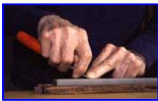
Using one or two fingers of the left hand (more fingers for wider blades), press down on the back of the blade at the very tip. The bevel must touch the stone firmly (oil will squish out). With the right hand add gentle support but allow the left hand's downward pressure to dominate totally.
