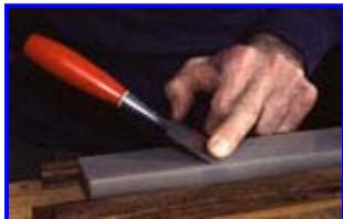
It is possible to hold the bevel flat against the honing stone with a single finger. While this is tiring and impractical, it does serve as the basis for a grip on the blade that will concentrate force at the bevel.
