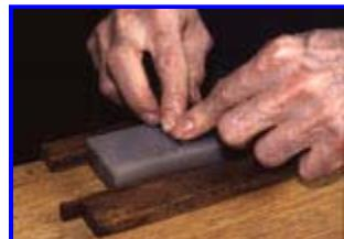
Be careful: if you run the handle of the tool onto the stone you can, accidentally, lift off the flat back off the cutting edge, spoiling its flatness.
