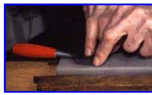
B: Rub bevel on Arkansas stone 10 - 20 strokes. This step is exactly like the previous bevel honing. The wire edge will flip over to the back.
