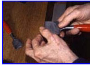
you hone the bevel the burr should be felt on the *back* side. As you flop back and forth, honing each side there will be less and less burr to be felt. Sometimes the burr drops off onto the stone, as a fine silver wire. When the burr is gone, you are done. Congratulations!
