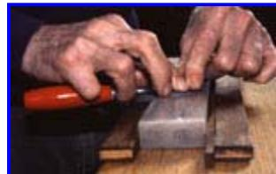
Notice how, while honing the back, the pressure is placed on the front of the tool, near the edge. Nevertheless the tool remains *flat on its back* and we are not lifting up from the stone at all during this process.
